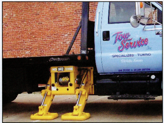
Rollback Sidewinder HD9000 is mounted underneath the bed and is rated at 9000lbs. Here it is in use position. The legs fold up when not in use.
