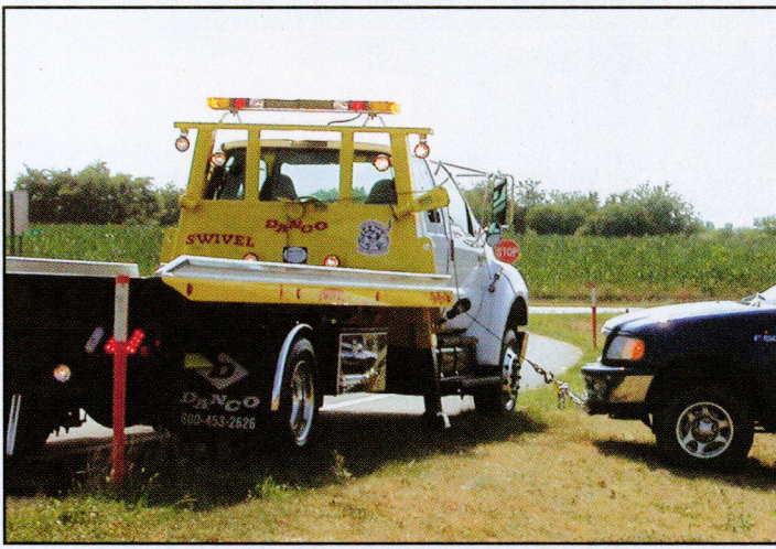
Danco's Sidewinding Cab Protector works off the winch on the main deck.
