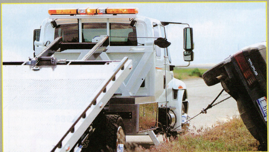
Miller Industries offers the Sidepuller in three configurations; SP8000, SP12000, and SP20000. Above an SP8000 at work.
