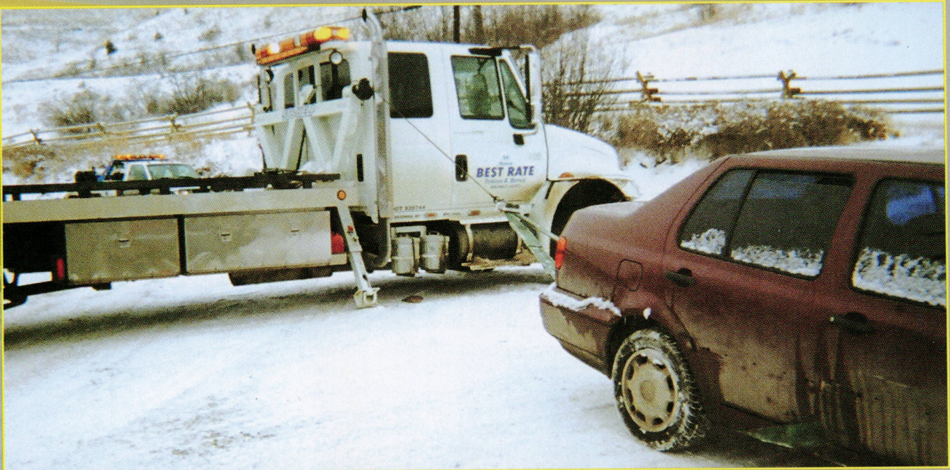
The SP8000 mounted on a carrier allows this unit to work off of the side as a recovery unit.
